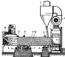
Direct rotary dryer: (1) cyclone, (2) blower, (3) product discharge chamber, (4) screw conveyor, (5) protruding rings, (6) support rollers, (7) drive, (8) girth gear, (9) spiral blades, (10) flights, (11) cylinder, and (12) feeder
