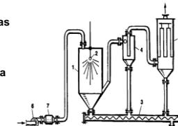
Spray dryer: (1) drying chamber, (2) atomizer, (3) screw conveyor for removing dried material, (4) cyclone, (5) bag filter, (6) blower, and (7) heater
